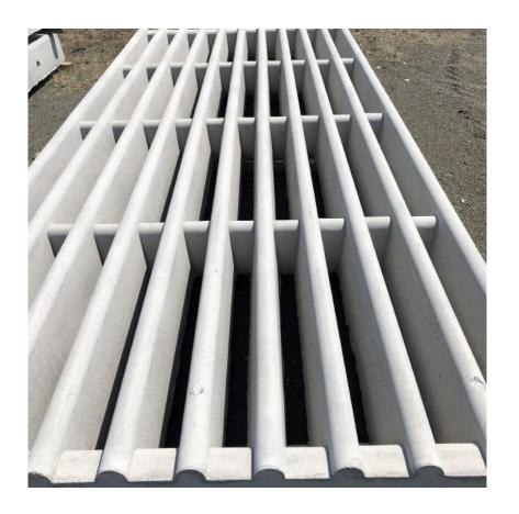
Our cattleguards are made of heavily reinforced concrete. It is precast in one piece and supports heavy machinery and truck loads. It is wider than other standard cattleguards and offers superior protection and durability. At the top of the cattleguard, the ribs are 3" and taper to 5" at the bottom, with 5' openings. All the top surfaces are rounded to reduce the possibility of edges chipping away. This design helps to ensure your cattleguard will last for years to come.
